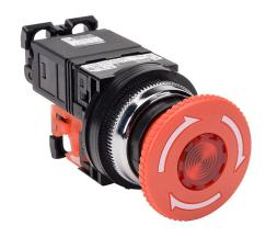
Fuji Electric emergency stop pushbutton, 30mm, twist-to-release, LED illuminated, (1) N.C. contact(s), plastic base, metal bezel, Operator: red, mushroom, 40mm, round, plastic, 115-127 VAC, transformer.
