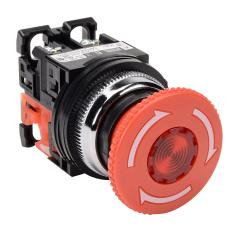
Fuji Electric emergency stop pushbutton, 30mm, twist-to-release, LED illuminated, (1) N.C. contact(s), plastic base, metal bezel, Operator: red, mushroom, 40mm, round, plastic, 24 VAC/VDC, full voltage.
