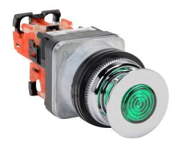
Fuji Electric pushbutton, 30mm, push-pull/momentary, LED illuminated, (1) N.O./(1) N.C. contact(s), plastic base, metal bezel, Operator: green, mushroom, 35mm, round, plastic, 24 VAC/VDC, full voltage.
