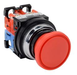
Fuji Electric emergency stop pushbutton, 30mm, push to lock, pull to reset, (1) N.O./(1) N.C. contact(s), plastic base, metal bezel, Operator: red, mushroom, 35mm, round, plastic.
