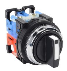
Fuji Electric selector switch, 30mm, 3-position, spring return from right to center / manual return from left to center, (1) N.O./(1) N.C. contact(s), plastic base, metal bezel, Operator: black, knob, 35mm, round, plastic.
