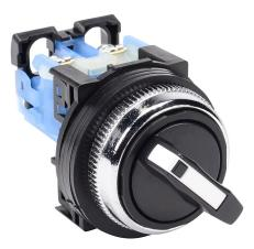
Fuji Electric selector switch, 30mm, 2-position, maintained, (1) N.O. contact(s), plastic base, metal bezel, Operator: black, knob, 35mm, round, plastic.
