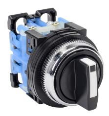
Fuji Electric selector switch, 30mm, 3-position, spring return from left and right to center, (2) N.O. contact(s), plastic base, metal bezel, Operator: black, knob, 35mm, round, plastic.
