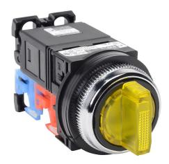
Fuji Electric selector switch, 30mm, 3-position, spring return from left to center / manual return from right to center, LED illuminated, (1) N.O./(1) N.C. contact(s), plastic base, metal bezel, Operator: yellow, knob, 35mm, round, plastic, 115-127 VAC, transformer.
