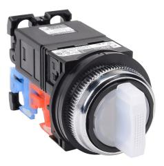
Fuji Electric selector switch, 30mm, 3-position, spring return from left to center / manual return from right to center, LED illuminated, (1) N.O./(1) N.C. contact(s), plastic base, metal bezel, Operator: white, knob, 35mm, round, plastic, 115-127 VAC, transformer.
