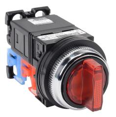
Fuji Electric selector switch, 30mm, 3-position, spring return from left to center / manual return from right to center, LED illuminated, (1) N.O./(1) N.C. contact(s), plastic base, metal bezel, Operator: red, knob, 35mm, round, plastic, 115-127 VAC, transformer.
