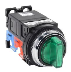
Fuji Electric selector switch, 30mm, 3-position, spring return from left to center / manual return from right to center, LED illuminated, (1) N.O./(1) N.C. contact(s), plastic base, metal bezel, Operator: green, knob, 35mm, round, plastic, 115-127 VAC, transformer.
