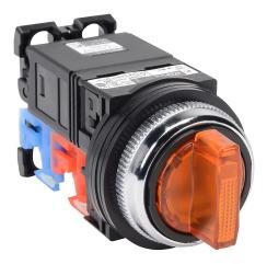
Fuji Electric selector switch, 30mm, 3-position, spring return from left to center / manual return from right to center, LED illuminated, (1) N.O./(1) N.C. contact(s), plastic base, metal bezel, Operator: orange, knob, 35mm, round, plastic, 115-127 VAC, transformer.
