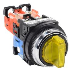
Fuji Electric selector switch, 30mm, 3-position, spring return from left to center / manual return from right to center, LED illuminated, (1) N.O./(1) N.C. contact(s), plastic base, metal bezel, Operator: yellow, knob, 35mm, round, plastic, 24 VAC/VDC, full voltage.
