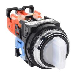
Fuji Electric selector switch, 30mm, 3-position, spring return from left to center / manual return from right to center, LED illuminated, (1) N.O./(1) N.C. contact(s), plastic base, metal bezel, Operator: white, knob, 35mm, round, plastic, 24 VAC/VDC, full voltage.
