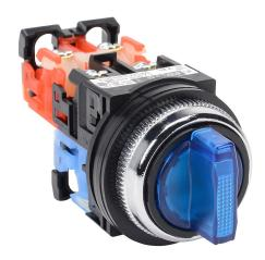
Fuji Electric selector switch, 30mm, 3-position, spring return from left to center / manual return from right to center, LED illuminated, (1) N.O./(1) N.C. contact(s), plastic base, metal bezel, Operator: blue, knob, 35mm, round, plastic, 24 VAC/VDC, full voltage.
