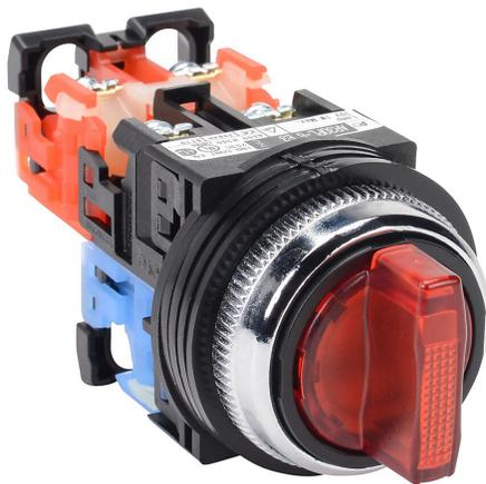
Fuji Electric selector switch, 30mm, 3-position, spring return from left to center / manual return from right to center, LED illuminated, (1) N.O./ (1) N.C. contact(s), plastic base, metal bezel, Operator: red, knob, 35mm, round, plastic, 24 VAC/VDC, full voltage.
