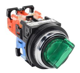
Fuji Electric selector switch, 30mm, 3-position, spring return from left to center / manual return from right to center, LED illuminated, (1) N.O./(1) N.C. contact(s), plastic base, metal bezel, Operator: green, knob, 35mm, round, plastic, 24 VAC/VDC, full voltage.
