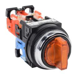
Fuji Electric selector switch, 30mm, 3-position, spring return from left to center / manual return from right to center, LED illuminated, (1) N.O./(1) N.C. contact(s), plastic base, metal bezel, Operator: orange, knob, 35mm, round, plastic, 24 VAC/VDC, full voltage.
