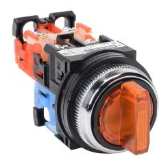
Fuji Electric selector switch, 30mm, 3-position, spring return from left to center / manual return from right to center, LED illuminated, (1) N.O./(1) N.C. contact(s), plastic base, metal bezel, Operator: orange, knob, 35mm, round, plastic, 24 VAC/VDC, full voltage.
