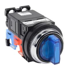
Fuji Electric selector switch, 30mm, 3-position, maintained, LED illuminated, (1) N.O./(1) N.C. contact(s), plastic base, metal bezel, Operator: blue, knob, 35mm, round, plastic, 115-127 VAC, transformer.
