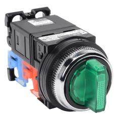
Fuji Electric selector switch, 30mm, 3-position, maintained, LED illuminated, (1) N.O./(1) N.C. contact(s), plastic base, metal bezel, Operator: green, knob, 35mm, round, plastic, 115-127 VAC, transformer.
