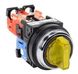
Fuji Electric selector switch, 30mm, 3-position, maintained, LED illuminated, (1) N.O./(1) N.C. contact(s), plastic base, metal bezel, Operator: yellow, knob, 35mm, round, plastic, 24 VAC/VDC, full voltage.
