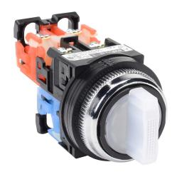
Fuji Electric selector switch, 30mm, 3-position, maintained, LED illuminated, (1) N.O./(1) N.C. contact(s), plastic base, metal bezel, Operator: white, knob, 35mm, round, plastic, 24 VAC/VDC, full voltage.
