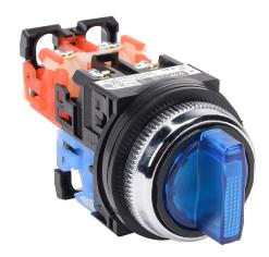
Fuji Electric selector switch, 30mm, 3-position, maintained, LED illuminated, (1) N.O./(1) N.C. contact(s), plastic base, metal bezel, Operator: blue, knob, 35mm, round, plastic, 24 VAC/VDC, full voltage.
