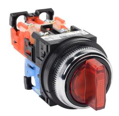
Fuji Electric selector switch, 30mm, 3-position, maintained, LED illuminated, (1) N.O./(1) N.C. contact(s), plastic base, metal bezel, Operator: red, knob, 35mm, round, plastic, 24 VAC/VDC, full voltage.
