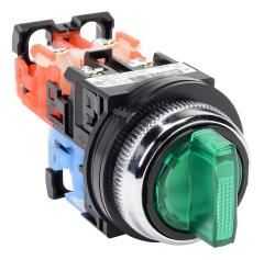
Fuji Electric selector switch, 30mm, 3-position, maintained, LED illuminated, (1) N.O./(1) N.C. contact(s), plastic base, metal bezel, Operator: green, knob, 35mm, round, plastic, 24 VAC/VDC, full voltage.
