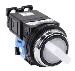
Fuji Electric selector switch, 30mm, 2-position, maintained, LED illuminated, (1) N.O. contact(s), plastic base, metal bezel, Operator: white, knob, 35mm, round, plastic, 115-127 VAC, transformer.
