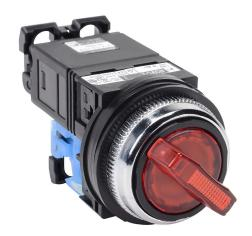
Fuji Electric selector switch, 30mm, 2-position, maintained, LED illuminated, (1) N.O. contact(s), plastic base, metal bezel, Operator: red, knob, 35mm, round, plastic, 115-127 VAC, transformer.
