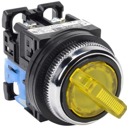
Fuji Electric selector switch, 30mm, 2-position, maintained, LED illuminated, (1) N.O. contact(s), plastic base, metal bezel, Operator: yellow, knob, 35mm, round, plastic, 24 VAC/VDC, full voltage.
