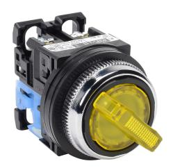
Fuji Electric selector switch, 30mm, 2-position, maintained, LED illuminated, (1) N.O. contact(s), plastic base, metal bezel, Operator: yellow, knob, 35mm, round, plastic, 24 VAC/VDC, full voltage.
