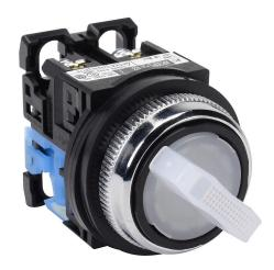
Fuji Electric selector switch, 30mm, 2-position, maintained, LED illuminated, (1) N.O. contact(s), plastic base, metal bezel, Operator: white, knob, 35mm, round, plastic, 24 VAC/VDC, full voltage.
