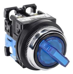
Fuji Electric selector switch, 30mm, 2-position, maintained, LED illuminated, (1) N.O. contact(s), plastic base, metal bezel, Operator: blue, knob, 35mm, round, plastic, 24 VAC/VDC, full voltage.
