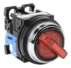
Fuji Electric selector switch, 30mm, 2-position, maintained, LED illuminated, (1) N.O. contact(s), plastic base, metal bezel, Operator: red, knob, 35mm, round, plastic, 24 VAC/VDC, full voltage.
