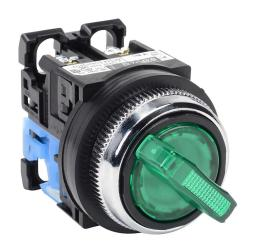
Fuji Electric selector switch, 30mm, 2-position, maintained, LED illuminated, (1) N.O. contact(s), plastic base, metal bezel, Operator: green, knob, 35mm, round, plastic, 24 VAC/VDC, full voltage.
