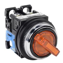
Fuji Electric selector switch, 30mm, 2-position, maintained, LED illuminated, (1) N.O. contact(s), plastic base, metal bezel, Operator: orange, knob, 35mm, round, plastic, 24 VAC/VDC, full voltage.
