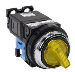
Fuji Electric selector switch, 30mm, 2-position, spring return from right, LED illuminated, (1) N.O. contact(s), plastic base, metal bezel, Operator: yellow, knob, 35mm, round, plastic, 115-127 VAC, transformer.
