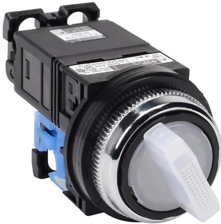
Fuji Electric selector switch, 30mm, 2-position, spring return from right, LED illuminated, (1) N.O. contact(s), plastic base, metal bezel, Operator: white, knob, 35mm, round, plastic, 115-127 VAC, transformer.
