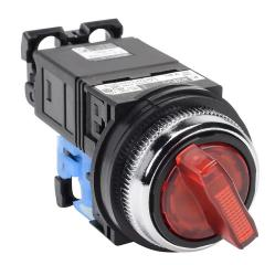
Fuji Electric selector switch, 30mm, 2-position, spring return from right, LED illuminated, (1) N.O. contact(s), plastic base, metal bezel, Operator: red, knob, 35mm, round, plastic, 115-127 VAC, transformer.
