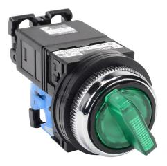
Fuji Electric selector switch, 30mm, 2-position, spring return from right, LED illuminated, (1) N.O. contact(s), plastic base, metal bezel, Operator: green, knob, 35mm, round, plastic, 115-127 VAC, transformer.
