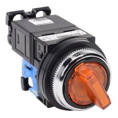
Fuji Electric selector switch, 30mm, 2-position, spring return from right, LED illuminated, (1) N.O. contact(s), plastic base, metal bezel, Operator: orange, knob, 35mm, round, plastic, 115-127 VAC, transformer.
