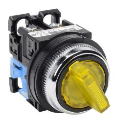
Fuji Electric selector switch, 30mm, 2-position, spring return from right, LED illuminated, (1) N.O. contact(s), plastic base, metal bezel, Operator: yellow, knob, 35mm, round, plastic, 24 VAC/VDC, full voltage.
