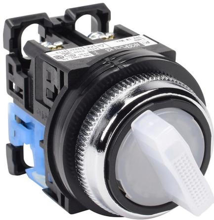
Fuji Electric selector switch, 30mm, 2-position, spring return from right, LED illuminated, (1) N.O. contact(s), plastic base, metal bezel, Operator: white, knob, 35mm, round, plastic, 24 VAC/VDC, full voltage.
