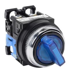
Fuji Electric selector switch, 30mm, 2-position, spring return from right, LED illuminated, (1) N.O. contact(s), plastic base, metal bezel, Operator: blue, knob, 35mm, round, plastic, 24 VAC/VDC, full voltage.
