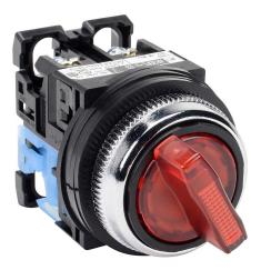
Fuji Electric selector switch, 30mm, 2-position, spring return from right, LED illuminated, (1) N.O. contact(s), plastic base, metal bezel, Operator: red, knob, 35mm, round, plastic, 24 VAC/VDC, full voltage.
