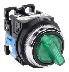
Fuji Electric selector switch, 30mm, 2-position, spring return from right, LED illuminated, (1) N.O. contact(s), plastic base, metal bezel, Operator: green, knob, 35mm, round, plastic, 24 VAC/VDC, full voltage.
