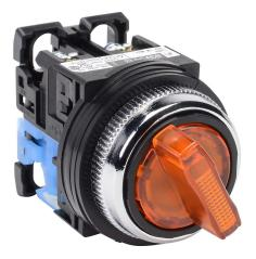
Fuji Electric selector switch, 30mm, 2-position, spring return from right, LED illuminated, (1) N.O. contact(s), plastic base, metal bezel, Operator: orange, knob, 35mm, round, plastic, 24 VAC/VDC, full voltage.
