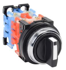
Fuji Electric selector switch, 30mm, 5-position, maintained, (2) N.O./(2) N.C. contact(s), plastic base, metal bezel, Operator: black, knob, 35mm, round, plastic.
