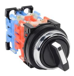
Fuji Electric selector switch, 30mm, 4-position, maintained, (2) N.O./(2) N.C. contact(s), plastic base, metal bezel, Operator: black, knob, 35mm, round, plastic.
