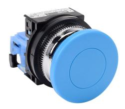
Fuji Electric pushbutton, 30mm, momentary, (1) N.O. contact(s), plastic base, metal bezel, Operator: blue, mushroom, 40mm, round, plastic.
