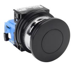
Fuji Electric pushbutton, 30mm, momentary, (1) N.O. contact(s), plastic base, metal bezel, Operator: black, mushroom, 40mm, round, plastic.
