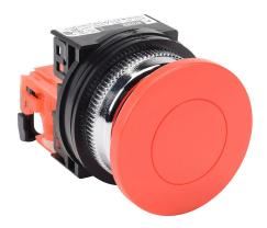
Fuji Electric pushbutton, 30mm, momentary, (1) N.C. contact(s), plastic base, metal bezel, Operator: red, mushroom, 40mm, round, plastic.
