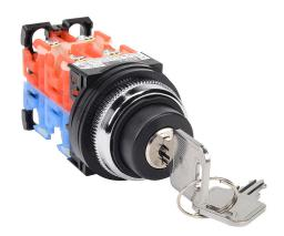
Fuji Electric selector switch, 30mm, 3-position, maintained, key removable left, right and center position, (2) N.O./(2) N.C. contact(s), plastic base, metal bezel, Operator: black, key, 35mm, round, plastic.
